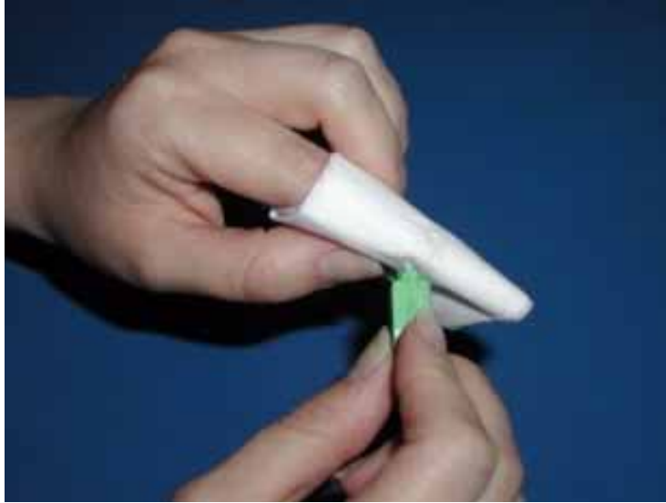
Figure 19 Wiping the connector with a Kim wiper
