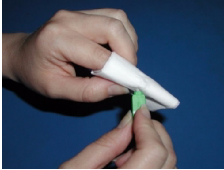
Figure 19 Wiping the connector with a Kim wiper
